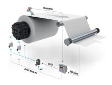
Combined regulation in torque with load cells or dancer roller
